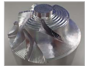
Breakage during machining
